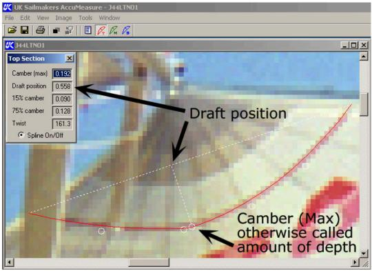
**Figure 2: FInding Max Camber and Draft Position**
